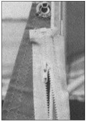
Start the zipper around forestay wire and jib halyard line. The jib halyard is internal in the luff of jib.
