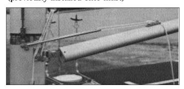
Tie rotator line 3/16" x 5') to fairlead built into the aluminum clam cleat, down through the eye in the rotator wishbone and back through the cleat. This provides a 2:1 purchase for adjusting mast rotation. 45 to 75 degrees rotation is considered normal for
