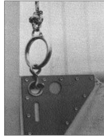
Attach the twisted shackle to the head of the mainsail and place forward edge of sail into curf of mast.
