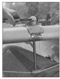
Loosen screw at bottom of striker rod.
